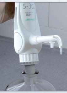
**Ground adapter for direct reagent extraction from a ground bottle** The NS 29/32 ground adapter enables secure use of the basic unit on standard ground bottles.
